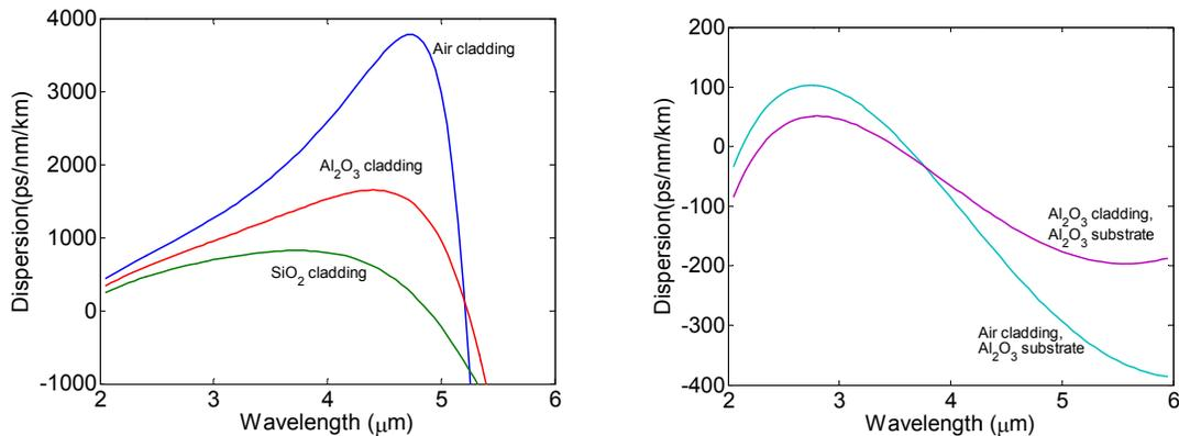
Figure 5. (a) The calculated dispersion of channel waveguide with air, sapphire and  $\text{SiO}_2$  as cladding materials. (b) Dispersion for rib/ridge waveguide with sapphire substrate and air and sapphire cladding.
