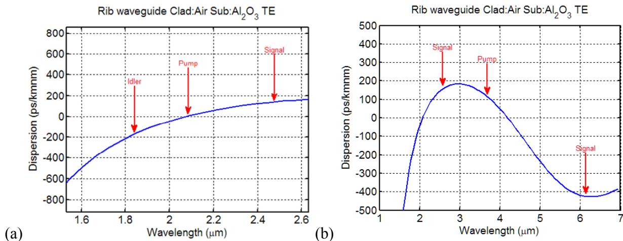
Figure 7. Phase matching concept of (a) conventional phasematching and (b) discrete band phase matching.
