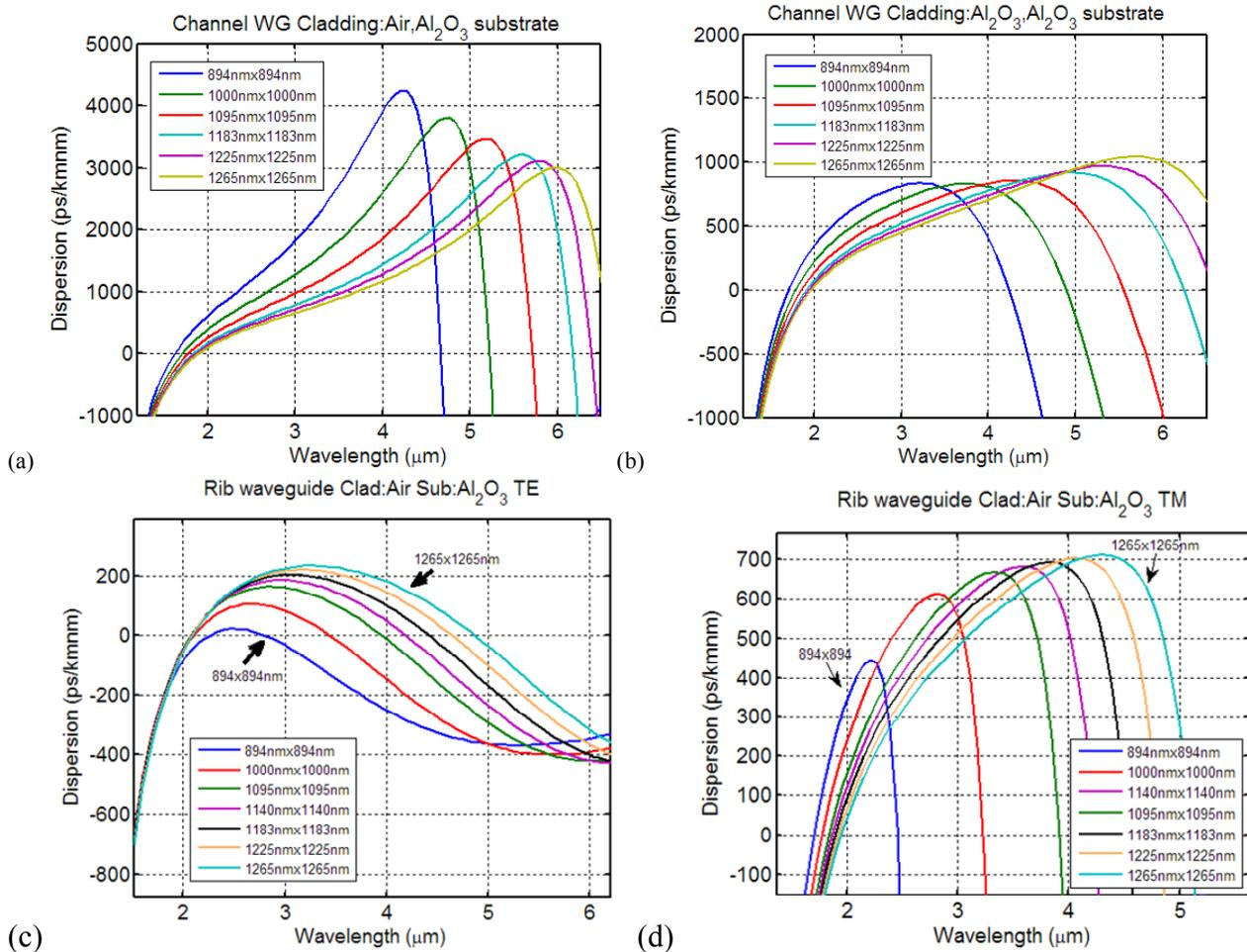
Figure 6. Dispersions of the channel waveguide surrounded by (a)air and (b) Sapphire and rib waveguide on sapphire with air cladding for (c)TE and (d)TM mode.
