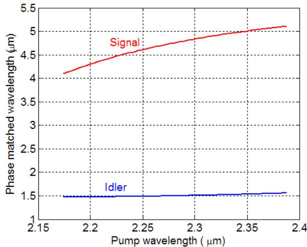
Figure 11. Phase matching condition for  $1\mu\text{m}$  by  $1\mu\text{m}$  rib waveguide with  $500\text{nm}$  slab region. Pump power is set at  $0.1\text{GW}/\text{cm}^2$ .
