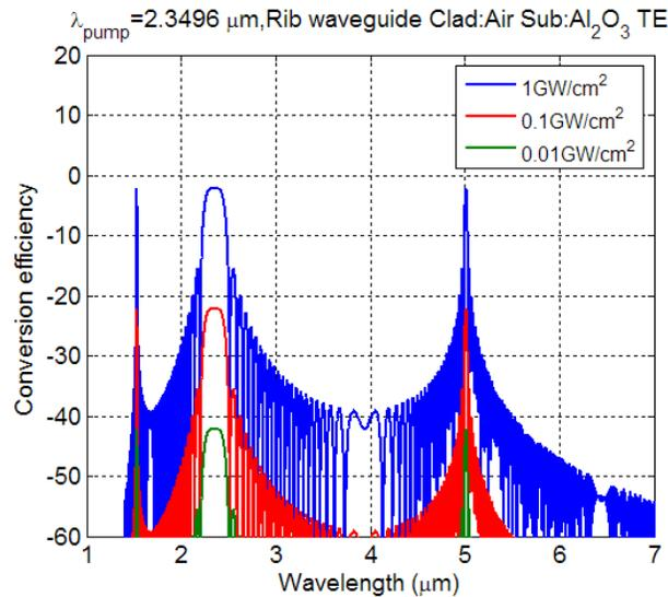
Figure 10. Conversion efficiency for  $1\text{GW}/\text{cm}^2$ ,  $0.1\text{GW}/\text{cm}^2$  and  $0.01\text{GW}/\text{cm}^2$  pump intensity at  $2.4\mu\text{m}$ . the maximum conversion efficiency is  $0\text{dB}$ ,  $-20\text{dB}$  and  $-40\text{dB}$ , respectively.
