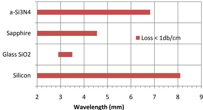
Figure 1. 1dB/cm transmission spectrum of the materials for MWIR silicon devices.
