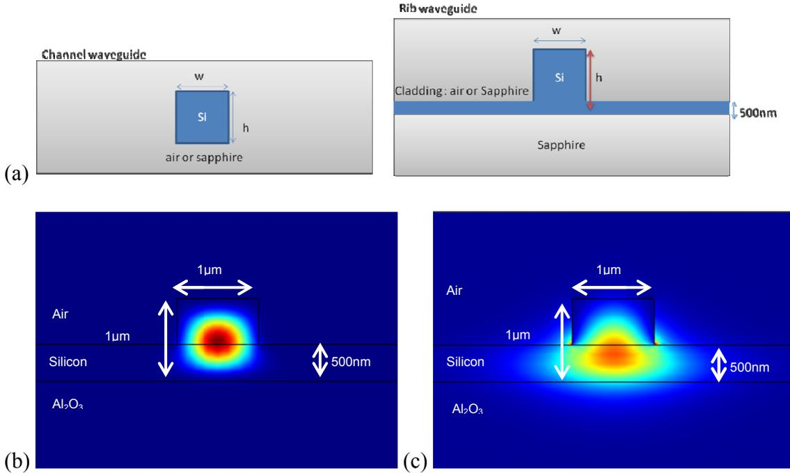
Figure 4. (a) The proposed waveguide structure and the mode profiles of the rib waveguide at (b)  $2\mu\text{m}$  and (c)  $5\mu\text{m}$ .
