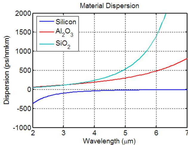
Figure 3. Material dispersion of silicon, sapphire,  $\text{SiO}_2$  and silicon nitride.
