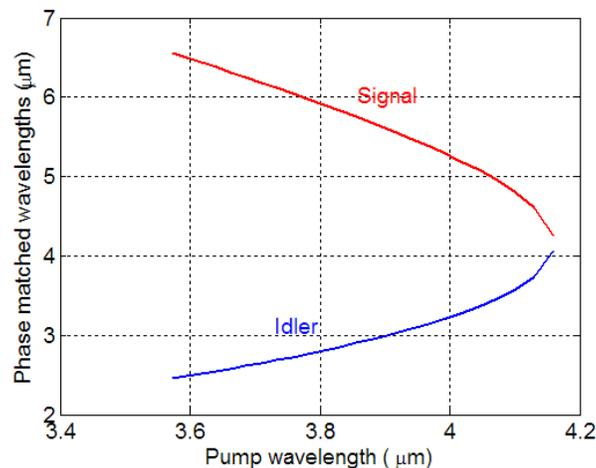
Figure 9. Phase matching wavelengths ( $\Delta k=0$ ) for rib waveguide with 500nm slab region. Pump power is set at  $0.1 \text{ GW/cm}^2$ .
